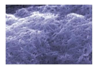
Scanning electron microscope image of "cleaned" carbon nanotubes at NIST (color added for clarity.) Credit: NIST
