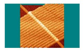
17 memristors in a row are visible on this AFM image. The memristor consists of two titanium dioxide layers connected to wires. When a current is applied to one, the resistance of the other changes. That change can be registered as data. Image credit: J.J. Yang / HP Labs
