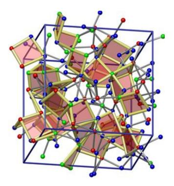
A model of an amorphous form of the memory material  $Ge_2Sb_2Te_5$ , showing the square molecular rings that nucleate the crystallization process.
