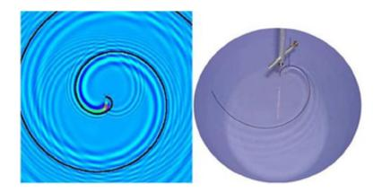
These diagrams show the surface deformation of water due to an object moving at 21 cm/s (0.9 times the minimum wave velocity) in a circular motion. Credit: Chepelianskii, et al.
