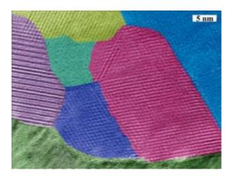
A cross-section of nano-crystalline bismuth antimony telluride grains, as viewed through transmission electron microscope. Colors highlight the features of each grain of the semiconductor alloy in bulk form. A team of researchers from Boston College and MIT produced a major increase in thermoelectric efficiency after using nanotechnology to structure the material, which is commonly used in industry and research. Credit: Boston College, MIT and GMZ Inc.
