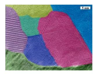
A cross-section of nano-crystalline bismuth antimony telluride grains, as viewed through transmission electron microscope. Colors highlight the features of each grain of the semiconductor alloy in bulk form. A team of researchers from Boston College and MIT produced a major increase in thermoelectric efficiency after using nanotechnology to structure the material, which is commonly used in industry and research. Credit: Boston College, MIT and GMZ Inc.
