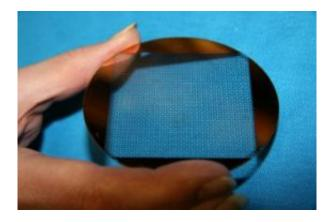
NIST researchers have made metafilms of tiny copper squares etched on a wafer. Credit: C. Holloway/NIST
