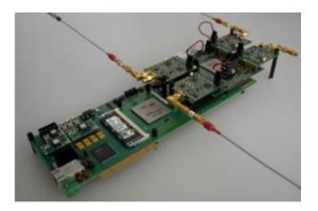
A prototype of a MIMO station with four antennas. 25cm high by 12cm wide. Credit: Photo: Group Prof. Boelcskei/ETH Zurich
