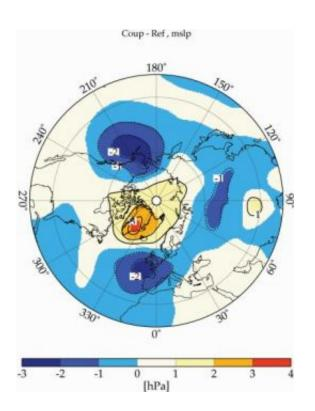
Difference of the sea level pressure between simulations with the new model including interactive stratospheric ozone chemistry relative to the standard model. There is an increase of air pressure above the Arctic (positive difference) and a decrease of air pressure in mid-latitudes (negative difference). This pattern is similar to the air pressure pattern of the negative phase of the Arctic Oscillation. Credit: Sascha Brand / Alfred Wegener Institute
