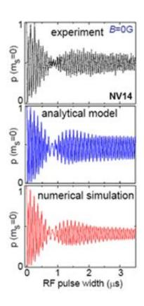
These images depicting coherently driven spin oscillations of a nitrogen-vacancy (N-V) center show the excellent level of agreement achieved between experiment, analytical theory and computer simulation in the research on the fundamental physics of a single quantum spin by Ames Laboratory, the University of California, Santa Barbara, and Microsoft Station Q.
