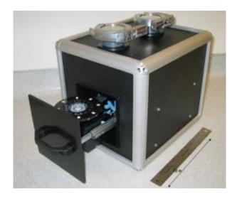
This prototype of the PANTHER device is about one cubic foot and weighs 37 pounds. Photo courtesy / MIT Lincoln Laboratory
