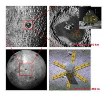
The crater Tsiolkovsky is a relatively level region on the far side of the Moon. A lander would deposit a series of rovers, which would then move out and unroll a set of arms containing individual antennas. The astronomical signals picked up by the antennas would be transmitted to back to the central lander for processing. Credit: NRL
