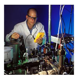
NIST physicist Till Rosenband adjusts the quantum logic clock, which derives its "ticks" from the natural vibrations of an aluminum ion (electrically charged atom). The aluminum ion is trapped together with one beryllium ion inside the copper-colored chamber in the foreground. Credit: Copyright Geoffrey Wheeler
