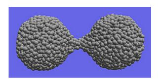
NIST researchers have shown that substances such as silica that are brittle in bulk exhibit ductile behavior at the nanoscale. Computer simulations demonstrate the material extension and necking that occurs during the separation of amorphous (top) and crystalline (bottom) silica nanoparticles. Credit: NIST
