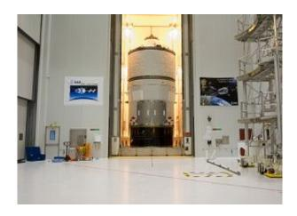
Jules Verne ATV is moved inside a special container (the CCU) to the Final Assembly Building (BAF) at Europe's Spaceport in Kourou, French Guiana, where the spacecraft will be finally integrated with the launcher. The Ariane 5 ES will lift ESA's first Automated Transfer Vehicle (ATV) into orbit. ATV will bring new supplies to the International Space Station. It will also be used to reboost the Station's orbit. (14 February 2008) Credits: 2008 - ESA /CNES/Arianespace/Photo optique video du CSG
