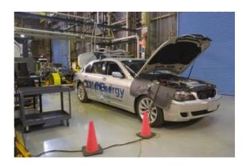
The BMW Hydrogen 7 Mono-Fuel demonstration vehicle, a near-zero emissions car, undergoes testing at Argonne&acutes Advanced Powertrain Research Facility (APRF), the principal U.S. Department of Energy facility for assessing advanced hybrid electric vehicle technologies. APRF is a unique facility in North America because it is the able to detect trace levels of emissions.
