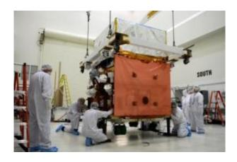
In the Astrotech payload processing facility, General Dynamics technicians watch as GLAST is moved toward a work stand (left) to check GLAST's scientific instruments. Credit: NASA/Kim Shiflett
