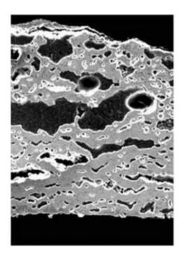
Conventional ceramic coating destroyed by molten glass. The field of view is about half a millimeter. Image by Aysegul Aygun and Nitin Padture, courtesy of Ohio State University
