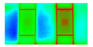
Infrared image of the outside wall of the control and test rooms. The test room, on the left, has undergone modifications. Its image shows significantly more blue (a colder temperature, less heat loss). The unmodified control room on the right shows little blue and much more green, orange and red colors that represent the warm air escaping to the outside. Credit: NIST
