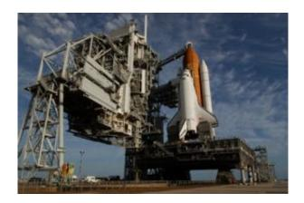
The rotating service structure is rolled back from around space shuttle Endeavour Monday morning. The enclosed gantry gives workers access to the shuttle and its payload bay leading up to launch. Credit: NASA
