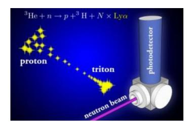
Neutron absorption by 3He yields tens of Lyman alpha photons, which result from the most fundamental energy jump in the hydrogen atom. This schematic illustrates the operation of a prototype Lyman alpha neutron detector. Credit: NIST
