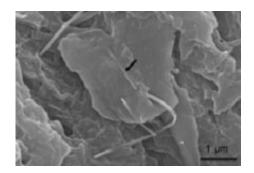
Field-emission scanning electron microscopy image of tissue sections obtained four weeks after CNTs were implanted into tibial defects in mice. CNTs (arrow) were integrated directly into the new bone and adhered closely to the bone matrix with no intervening space. Credit: Small, 2008
