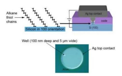
Side and top views of the NIST molecular resistor. Above are schematics showing a cross-section of the full device and a close-up view of the molecular monolayer attached to the CMOS-compatible silicon substrate. Below is a photomicrograph looking down on an assembled resistor indicating the location of the well. Credit: NIST
