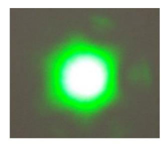
The researchers used ultrashort light pulses in microstructured optical fibres to demonstrate the formation of an artificial event horizon. This image captures the light at the end of the optical fibres (Photo: Chris Kuklewicz)
