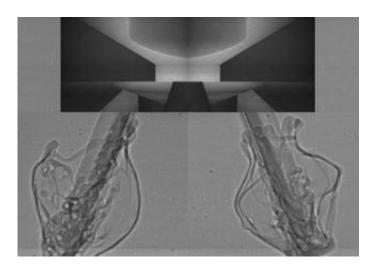
The liquid breakup of a high density stream from a fuel injector can easily be seen using an X-ray technique developed at Argonne National Laboratory. The technique could lead to better and cleaner fuel injectors.
