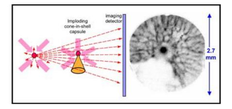
This schematic drawing shows the system MIT physicists are using to study tiny implosions of hydrogen fuel. On the left, protons streaming away from the farleft implosion travel through magnetic and electric fields generated by the other implosion. On the right is the resulting image of the fields, with the compressed hydrogen pellet in the center. Image courtesy / Richard Petrasso
