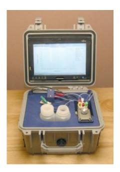
PNNL's biomonitoring detection system uses two classes of sensors to analyze blood, urine or saliva samples. While small and portable, the sensitive system provides detection levels at parts-per-billion. Credit: PNNL
