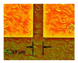
Optical micrographs of typical FET structures in the NIST/Penn State/UK experiments show the effect of pretreating contacts to promote organic crystal formation. Treated structure (1) shows crystal structure extending from the rectangular contacts and merging in the channel in contrast to untreated contacts (r). Credit: NIST
