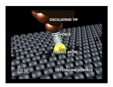
Illustration of an Atomic Force Microscope (AFM) tip measuring the force it takes to move a cobalt atom on a crystalline surface. The ability to measure the exact force it takes to move individual atoms is one of the keys to designing and constructing the small structures that will enable future nanotechnologies. Credit: IBM
