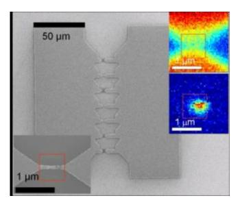
Rice University scientists used tiny gaps in narrow gold wires to simultaneously capture electronic and optical measurements of the same molecule. These scanning electron images show the wires and gaps. The color insets are maps of optical signals from the gap. Credit: D. Natelson/Rice University
