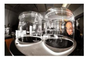
Hy Tran examines a kilogram sample in a mass comparator at Sandia's Primary Standards Laboratory. Credit: Randy Montoya
