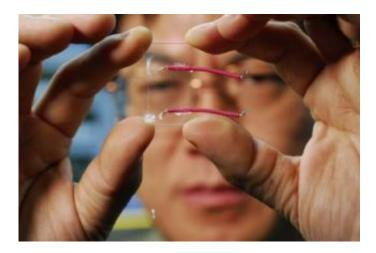
Georgia Tech Professor Zhong Lin Wang shows a microfiber nanogenerator composed of a pair of entangled fibers. Both fibers are coated with zinc oxide nanowires; one fiber is additionally coated with gold. When rubbed together, they generate electrical current. Credit: Georgia Tech Photo: Gary Meek
