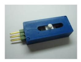
Non-contact position sensors are small but important parts of many modern machines. Researchers have used a phenomenon known as magnetoresistance to develop a practical, low-cost position sensor that performs better than existing designs. Commercial production will follow this year.
