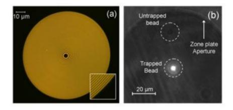
(a). Photograph of microfabricated Fresnel Zone Plate optical tweezer, consisting of concentric gold rings (50 nm thick) on a microscope slide. The Zone Plate outer diameter is 100<sup>1</sup>/4m, and the focal length is 8<sup>1</sup>/4m. (b). CCD camera image of fluorescent bead (2<sup>1</sup>/4m diameter) trapped in Zone Plate focus. Credit: Ken Crozier, Harvard School of Engineering and Applied Sciences
