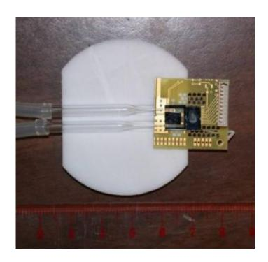
Prototype microchip device combining NIST's miniature atomic magnetometer with a fluid channel for studies of tiny samples. Credit: NIST
