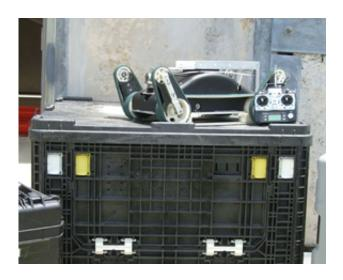
Urban search and rescue robot and its control unit sit atop one of the packing crates stipulated in a new ASTM International standard designed to help first responders manage storage and transportation logistics. Credit: NIST
