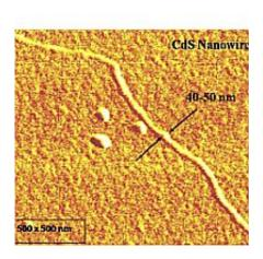
A section of nanowire produced by Texas A&M mechanical engineering researchers postdoctoral researcher Subrata Kundu and associate professor Hong Liang. The electrically conducting nanowire is about 1/1,000 the width of a human hair and could be used in developing nanoscale electronic devices.
