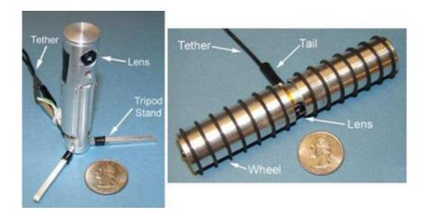
Two in vivo camera robots used by the Aquanauts during the NEEMO mission. Image credit: Rentschler, et al. ©IEEE 2008.
