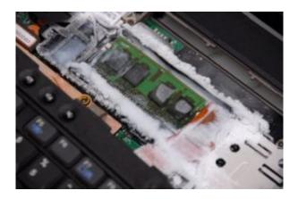
A combination of frost and refrigerant around the computer's memory chips. At this temperature, memory contents last for several minutes with almost no loss of information.
