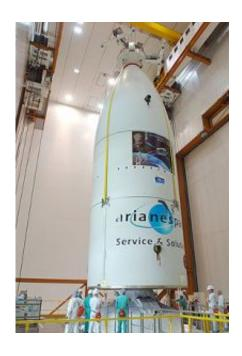
Jules Verne, the first Automated Transfer Vehicle, has been integrated and encapsulated under its huge fairing on top of its Ariane 5 launcher. With a total mass of about 19 360 kg, Jules Verne is the largest payload ever launched by Ariane 5. The historical mission with the first European space supplier for the ISS is scheduled for a night time launch on 8 March at 01:23 local time in French Guiana (04.23 UT). Credits: 2008 - ESA /CNES/Arianespace/Photo optique video du CSG
