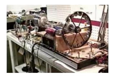
Thane Heins' "Perepiteia" generator seems to turn magnetic friction into a magnetic boost, causing the motor to accelerate in a positive feedback loop.
