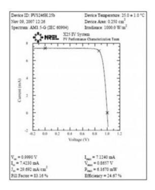
Performance characterization of IMEC's GaAs cell, measured by NREL.
