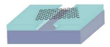
A schematic of a graphene sheet placed over a trench in a substrate.
