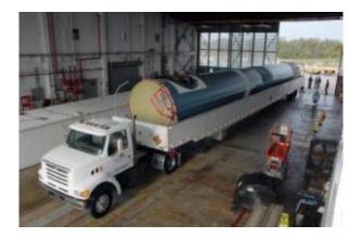
The United Launch Alliance Delta II rocket's first stage was revealed after the cover was removed from the truck that delivered it. It was delivered during the week of Feb. 4. Credit: NASA
