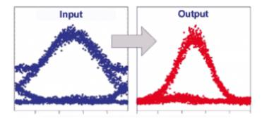
After traveling through 20 kilometers of optical fiber a pulse of light a few picoseconds long becomes distorted. "Pumping" with a clean pulse on a photonic microchip can sharpen the signal before sending it further down the line. Credit: Gaeta Lab
