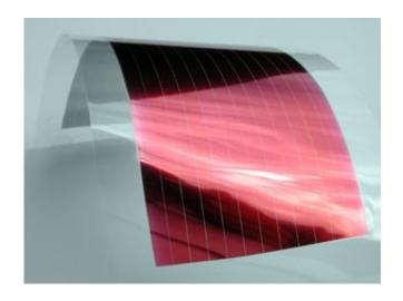
The flexible solar module is as small as the page of a book. © Fraunhofer ISE
