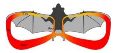
A simplified representation of the strong vortices associated with the unsteady aerodynamics of bat flight at slow speeds. The vortices can be thought of as causing the surrounding air to rotate rapidly around them and this motion around the LEV on top of the wing increases the lift force on it. Just like familiar, fixed-wing planes, the bat also leaves tip vortices in its wake, but the overall flow is further modified by the start vortices created at the beginning of the downstroke. Credit: USC
