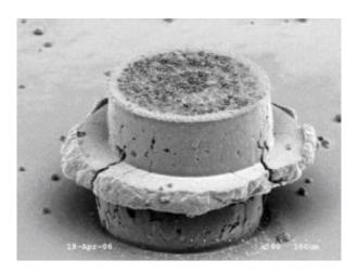
Scanning electron microscope image of two copper pillars bonded together using a novel fabrication technique. Placing these all-copper connections between computer chips and external circuitry will lead to increased computing speeds. Credit: Image courtesy of Tyler Osborn
