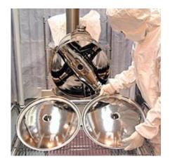
A superconducting triple-spoke cavity is prepared for electropolishing in a clean room. Argonne National Laboratory photo.
