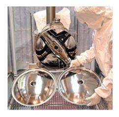
A superconducting triple-spoke cavity is prepared for electropolishing in a clean room. Argonne National Laboratory photo.
