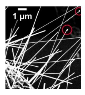
ZnO nanowires to grow out of the circular copper substrate in all directions, as seen in this scanning electron micrograph. Detail image shows copper droplets at the tip of some nanowires. Credit: NIST
