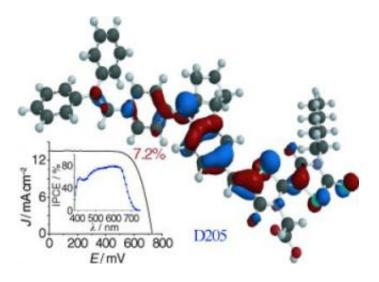
Current-voltage plot and photocurrent action spectrum for the sensitizer D205, the highest occupied molecular orbital of which is shown. (c) Wiley-VCH 2008
